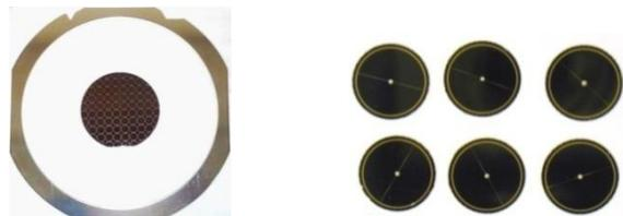
**Figure 9:** 100mm patterned wafer on dicing tape (left). Individual, fully plasma singulated devices with through wafer holes (right). (Courtesy Opto Diode an ITW company).
