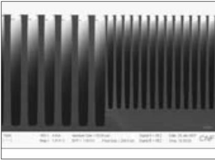
Figure 14. Run 3 conditions with an oxide mask depicting 10 $\mu$ m and 5 $\mu$ m features with a selectivity of 340:1 and an etch rate of 7 $\mu$ m/min
