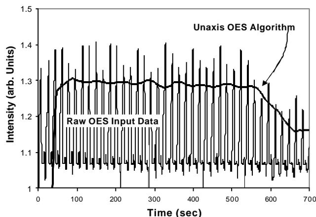
Figure 5: OES endpoint signal from SOI etching with 2% oxide exposed on 150-mm wafer.
