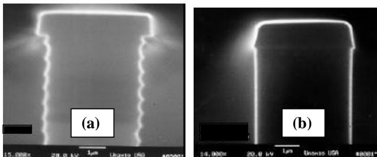
Figure 2: SEM images (a) sidewall scallops using conventional etching process. (b) smoother sidewalls using fast gas switching technique with an etching rate of  $>7 \mu\text{m}/\text{min}$ . The smoother sidewall with  $<35 \text{ nm}$  roughness is achieved at twice the etching rate in (a).
