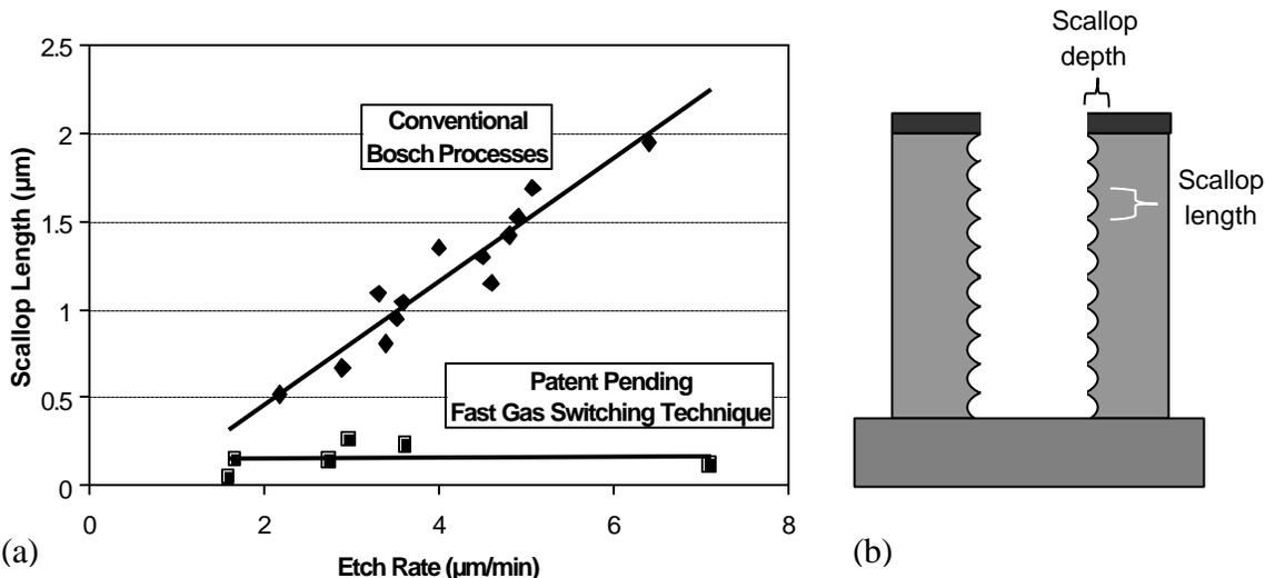
Figure 1: (a) Correlation between scallop length and etching rate with conventional etching processes and the small scallop length possible with high etching rates using new fast gas switching method. (b) scallop depth is related to scallop length.
