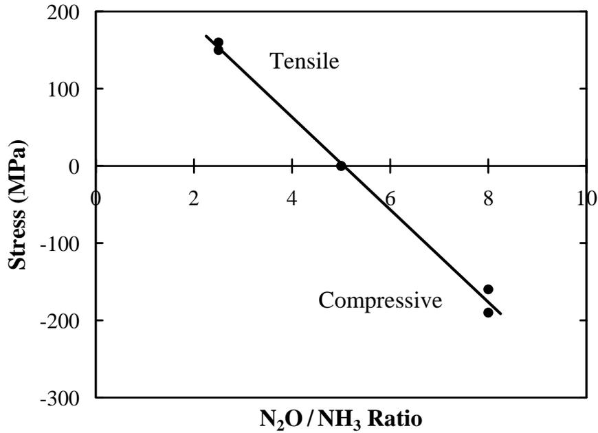
Figure 4. Variation of stress of PECVD  $SiO_yN_x$  films deposited at  $250^\circ C$  with  $N_2O/NH_3$  gas flow ratio. The deposition rates were about  $300 \text{ \AA}/\text{min}$ .
