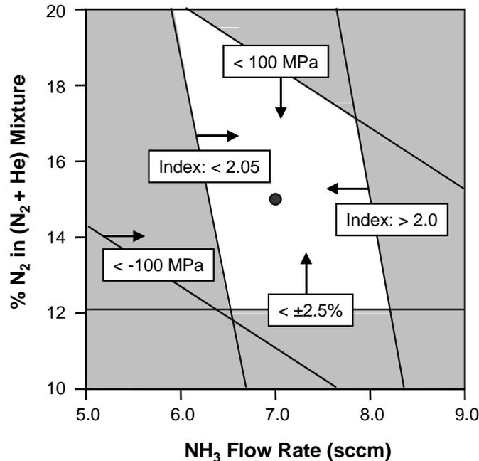
Figure 13. Overlay plot for an optimized 300°C low stress  $\text{SiN}_x$  process. Non-shaded area shows the optimized process regime. Point in center denotes the center point of the design.
