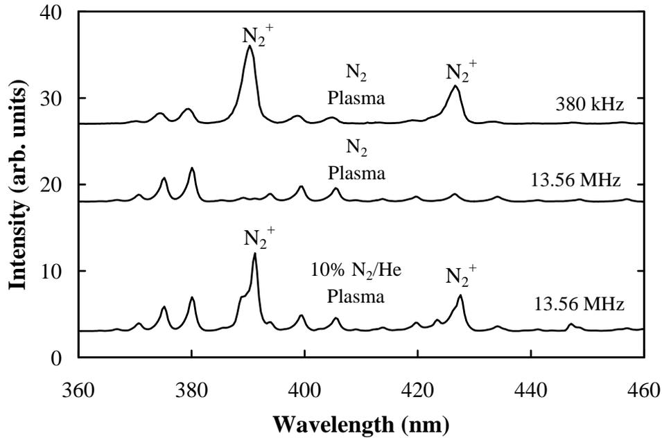
Figure 11. Optical Emission Spectra for 13.56 MHz plasmas of  $N_2$  and 10%  $N_2$  in He. Also shown is a spectra of a low frequency, 380 kHz  $N_2$  plasma. Spectra are displaced vertically for clarity.
