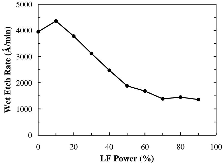
Figure 9. Variation of wet-etch rate of PECVD SiO<sub>2</sub> deposited at 350°C with added low-frequency power. The data refers to the same series of films used in Figure 7. For reference, the measured wet-etch rate of thermally grown SiO<sub>2</sub> is about 800 Å/min.
