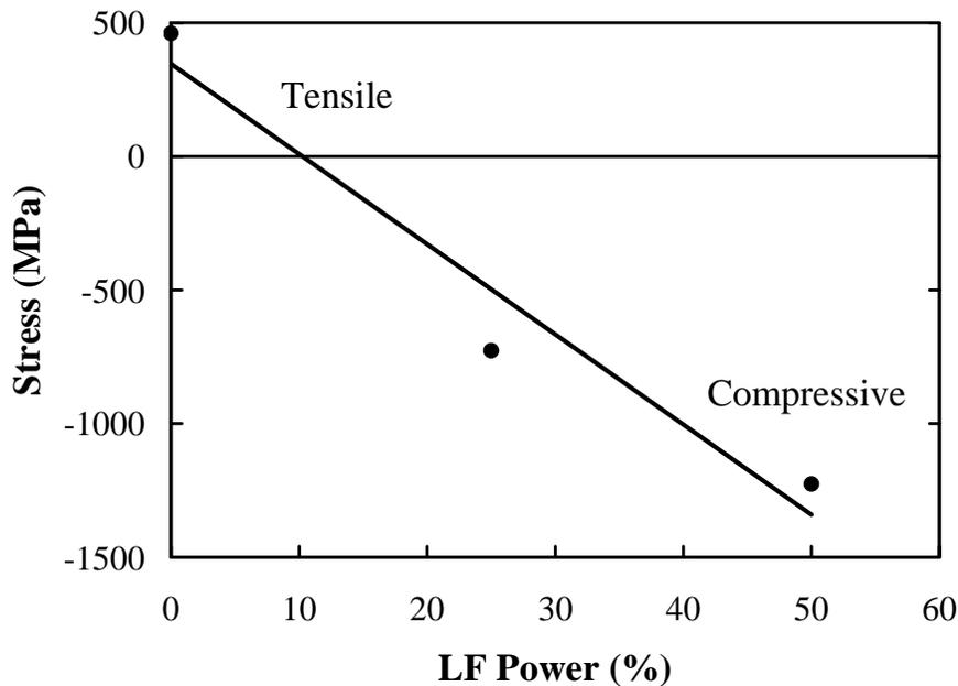
Figure 6. Stress of PECVD  $\text{SiN}_x$  films deposited at  $350^\circ\text{C}$  as a function of added low-frequency power. The deposition rates were between 500 and  $1000 \text{ \AA}/\text{min}$ .
