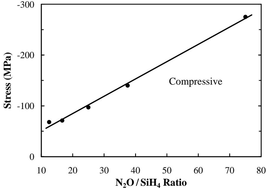
Figure 2. Stress of PECVD SiO<sub>2</sub> films deposited at 250°C as a function of N<sub>2</sub>O/SiH<sub>4</sub> gas flow ratio. The deposition rates were about 500 Å/min.
