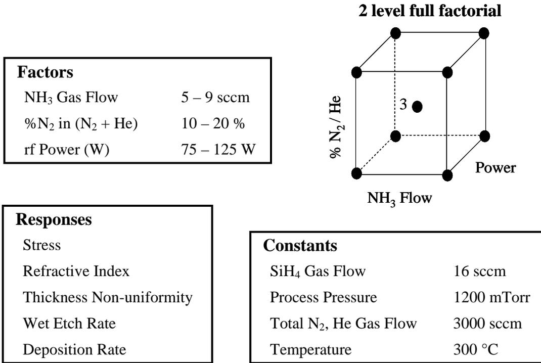
Figure 12. Factors, responses, and constants for the two level full factorial designed experiment for optimization of the low stress  $\text{SiN}_x$  process.
