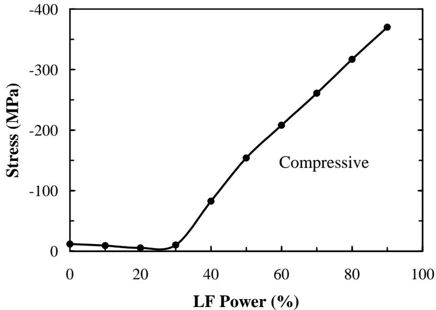
Figure 7. Stress of PECVD SiO<sub>2</sub> films deposited at 350°C as a function of added low-frequency power. The deposition rates were about 3000 Å/min.
