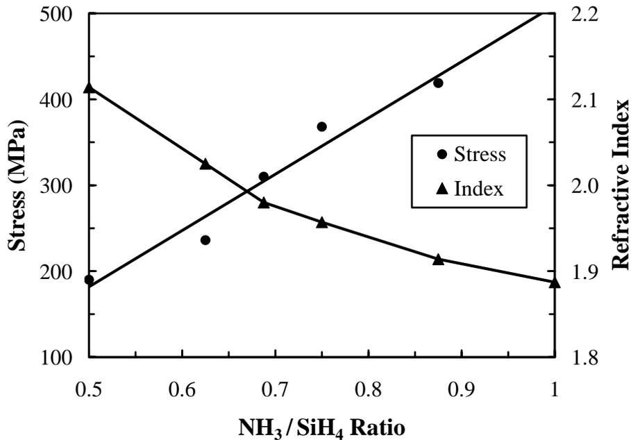
Figure 3. Tensile stress and refractive index of PECVD SiN<sub>x</sub> films deposited at 250°C as a function of NH<sub>3</sub>/SiH<sub>4</sub> gas flow ratio. Deposition rates were about 120 Å/min.
