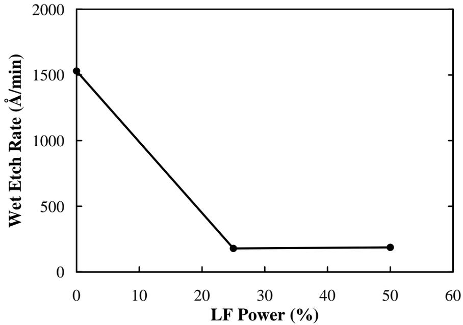
Figure 8. Variation of wet-etch rate of PECVD SiN<sub>x</sub> deposited at 350°C with added low-frequency power. The data refers to the same series of films used in Figure 6.
