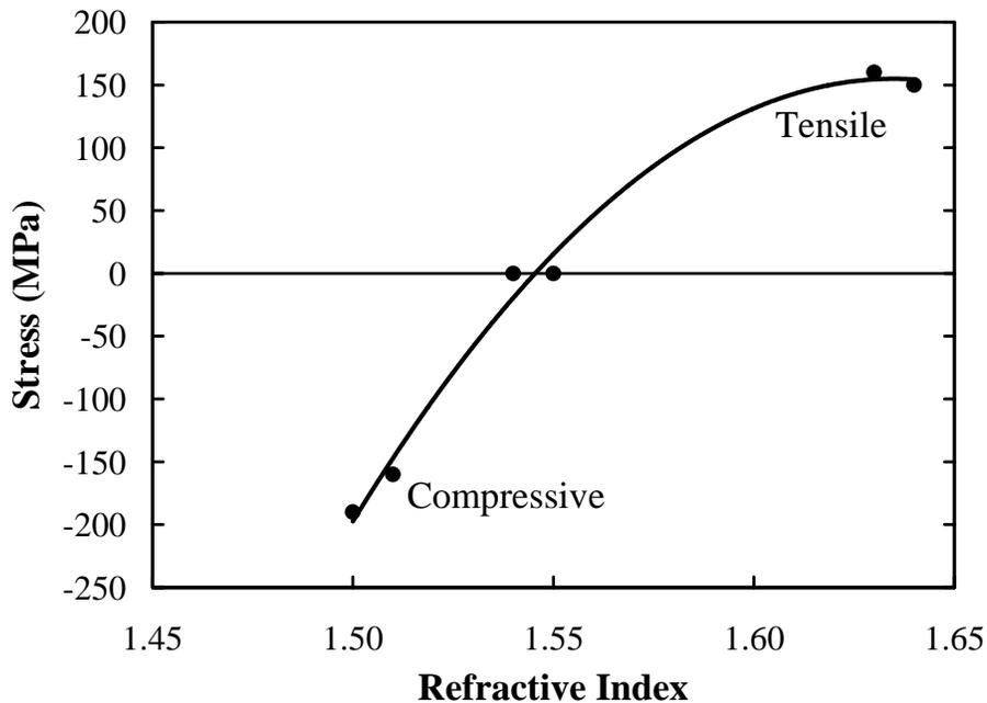
Figure 5. Stress of the PECVD  $SiO_yN_x$  films from Figure 4 *versus* refractive index.
