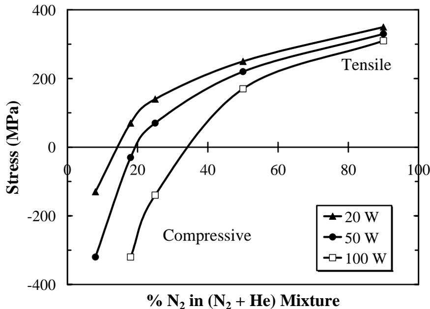
Figure 10. Stress control of PECVD SiN<sub>x</sub> by the He dilution method. The SiN<sub>x</sub> films were deposited at 250°C at the different rf power levels indicated in the figure. The deposition rates were about 120 Å/min.
