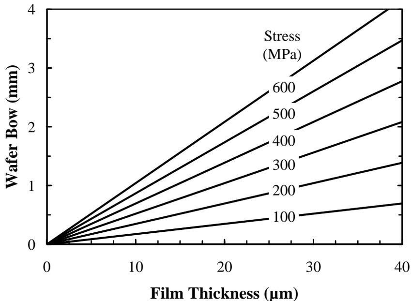
Figure 1. Calculated maximum bow of a 150 mm Si wafer *versus* deposited film thickness for the various film stress values indicated. (Bow estimated from Stoney's equation [11] using the parameters: wafer thickness 650  $\mu\text{m}$ , Poisson's ratio 0.22, and Young's modulus 180 GPa).
