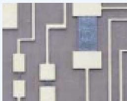
of 100% during operation and storage for 1000 hours at 150°C was assumed. The most stable region is between 50 Ohm/square to 200 Ohm/square.
