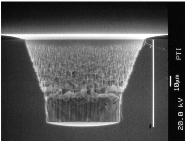
**Figure 3-Selective GaAs/AlGaAs Etch Result**
