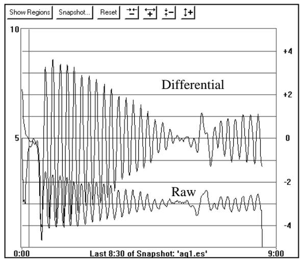
Figure 5. OES intensity as a function of etch time.
