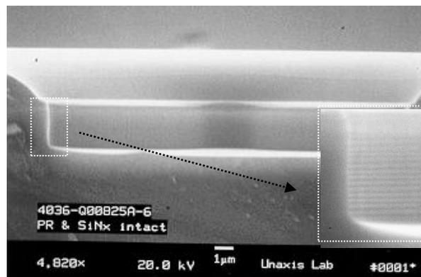
Figure 3. SEM photograph of VCSELs structure after etching with the optimized process; a vertical profile is observed.
