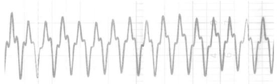
Figure 4. Laser reflectivity as a function of etch time.
