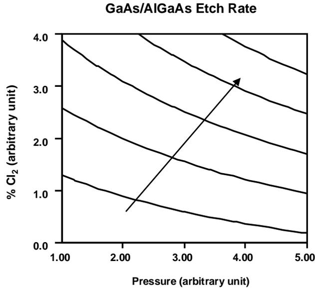
Figure 2. Contour plot of the GaAs/AlGaAs etch rate response surface as a function of pressure and Cl<sub>2</sub>%.
