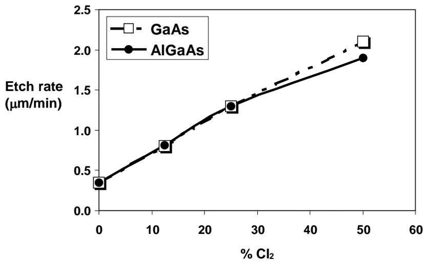
Figure 1. The etch rates of GaAs and AlGaAs as the function of the %Cl<sub>2</sub>
