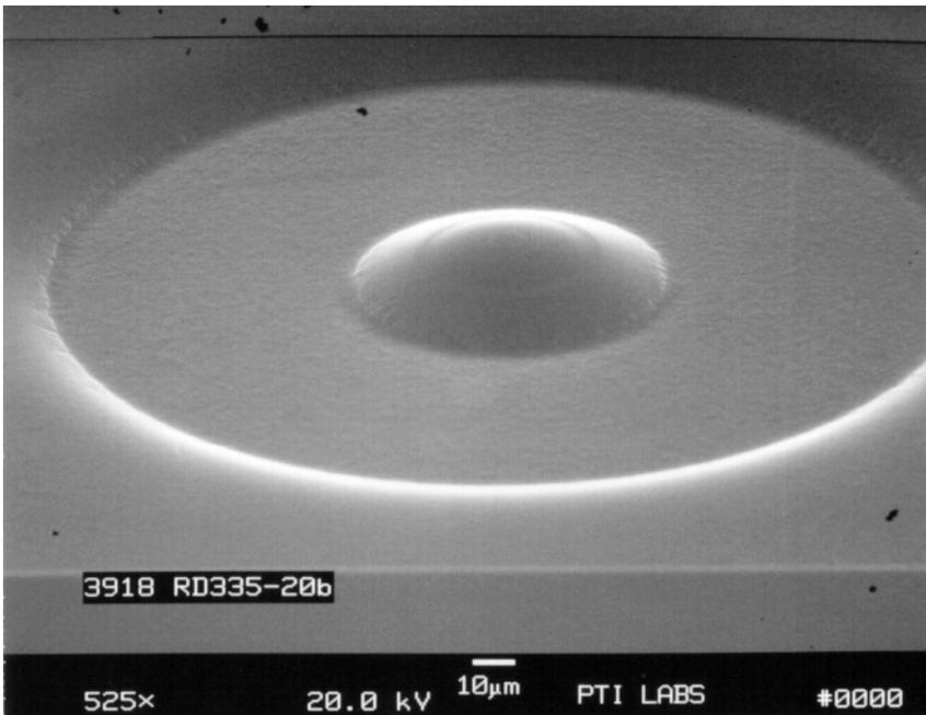
Figure 2. SEM photo of InP lens etched in an ICP plasma
