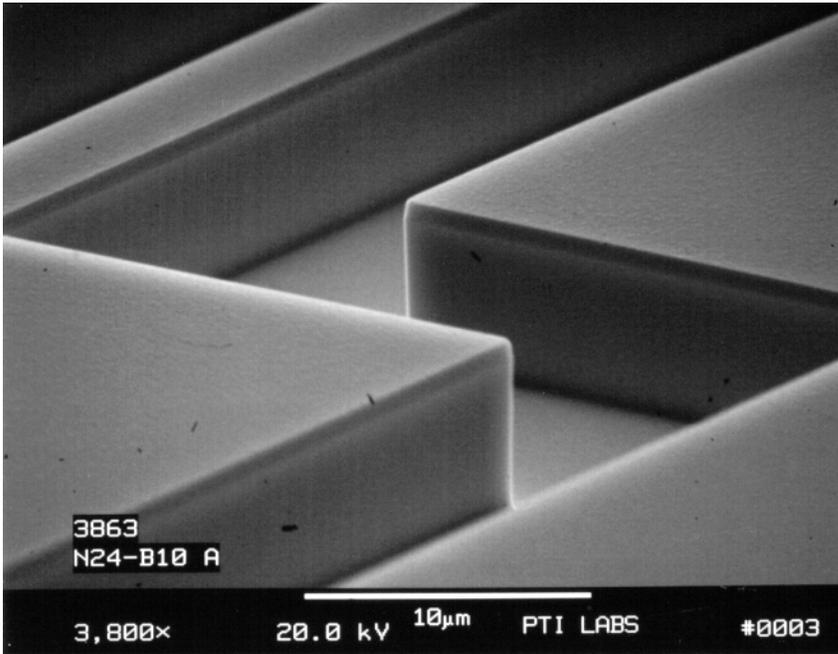
Figure 1. SEM photo of InP etched in an ICP plasma.
