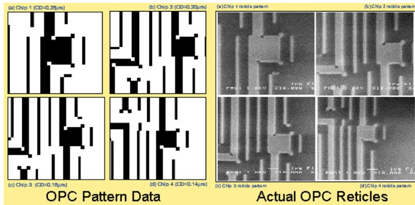
**OPC Serifs on the Photomask add light at the edges and corners of a feature when printed on the wafer**
