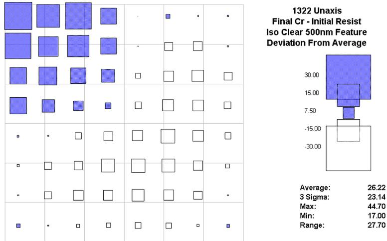
**Best “Gen 3” dry etch process shows very large Brightfield/Darkfield etch signature disparity in the clear (window) vs. the dark (outer) area.**
