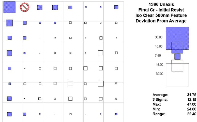
Initial “Gen 4” dry etch process shows almost no Brightfield/Darkfield etch signature disparity in the clear (window) vs. the dark (outer) area.
