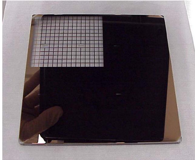
**Highly uneven pattern with >99% Cr load in window and <1% Cr load on remaining area.**
